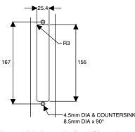
4. Drill appropiate holes to suit lockset to be fitted. Dimensions shown suit all functions. Note 23mm standard backset shown, others include 25.4mm, 30mm and 38mm.
